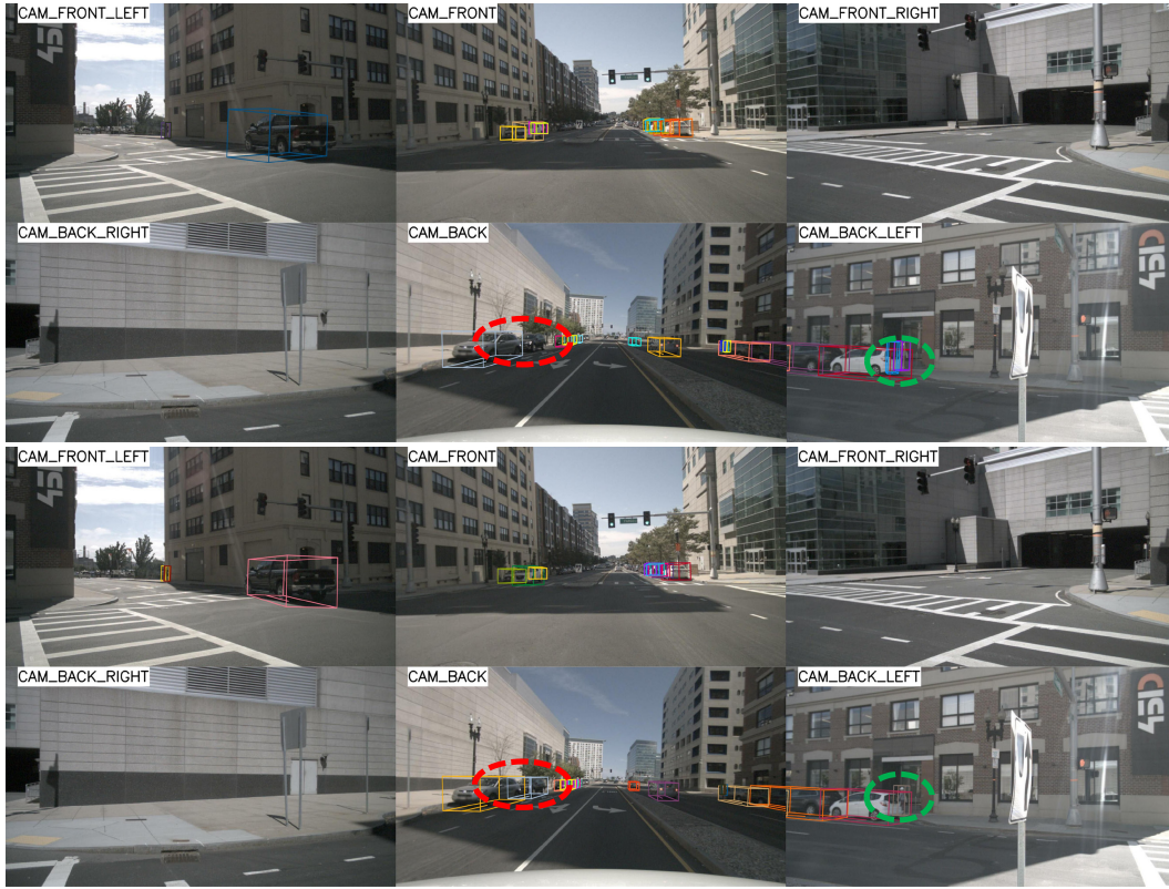
Figure 1: Visualization of 3D object detection results. The top and bottom two rows denote detection results of SparseBEV and ours, respectively. The false negatives and false positives are annotated with red dotted circles and green dotted circles, respectively.
